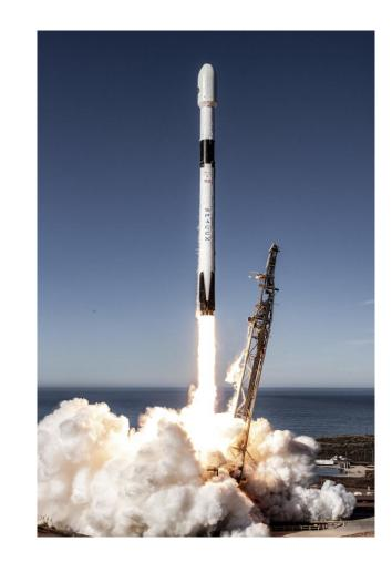
Falcon 9 can lift 22,800 kg payload mass to Low Earth Orbit, making it ideal for launching heavier satellites like GSAT-20.
